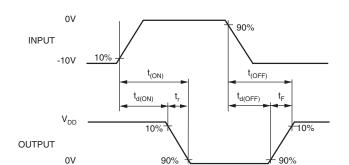
**Switching Waveform & Test Circuit**
